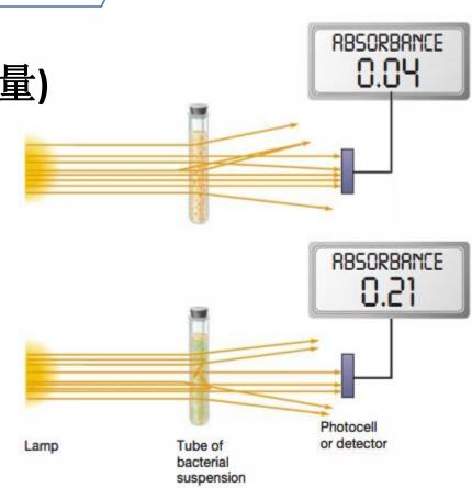
Figure 7.37 Turbidity and Microbial Mass Measurement.
